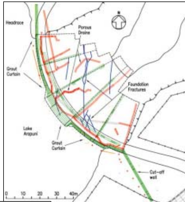
Figure 2. Plan view of Arapuni Dam. The positions of the foundation fractures noted during construction are shown. The diversion tunnel curves to the south of the right abutment cut-off wall.
