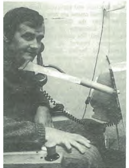
Injured in a car crash, this man can only move his head. A mouth stick for depressing a push-hook and for pushing the buttons on a decadic push-button phone, as well as a handset mounted on a flexible stand, enable him to operate the telephone independently.
