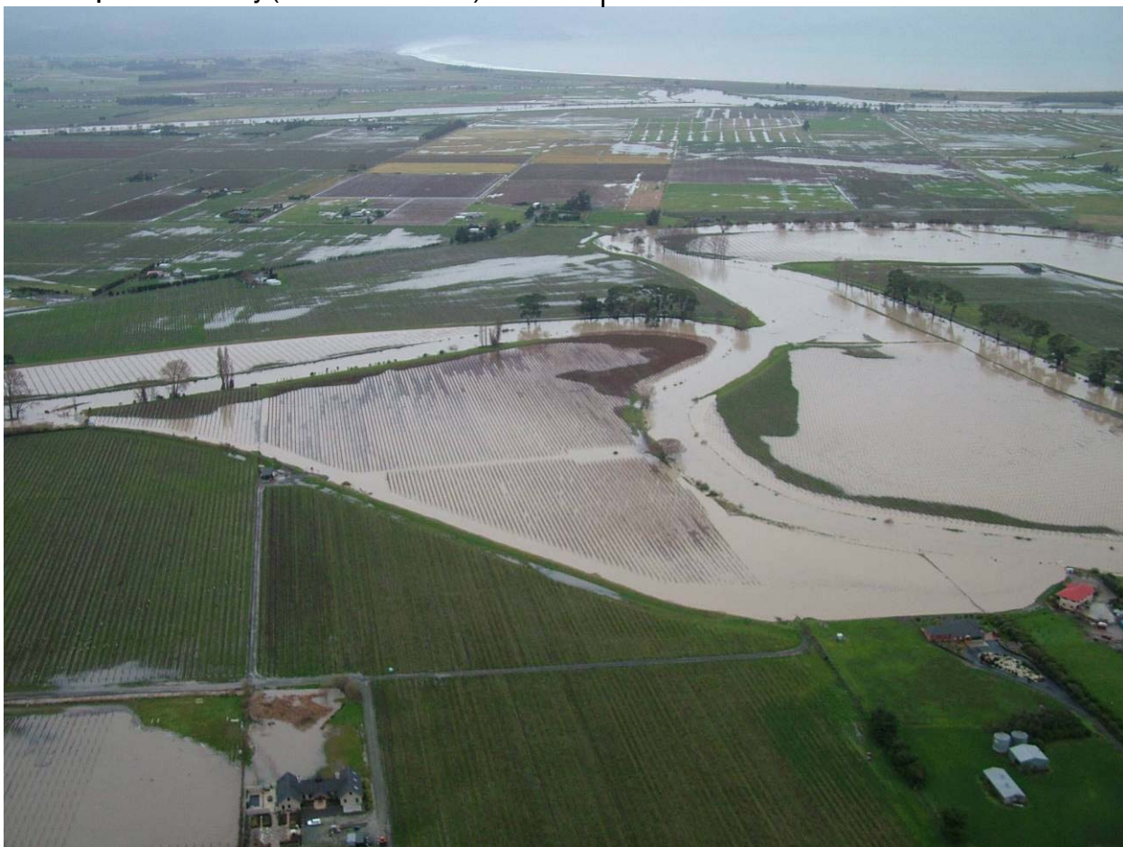
FIGURE 3: Complex channel and berm flow hydraulics of the Lower Opawa floodway in July 2008 flood
