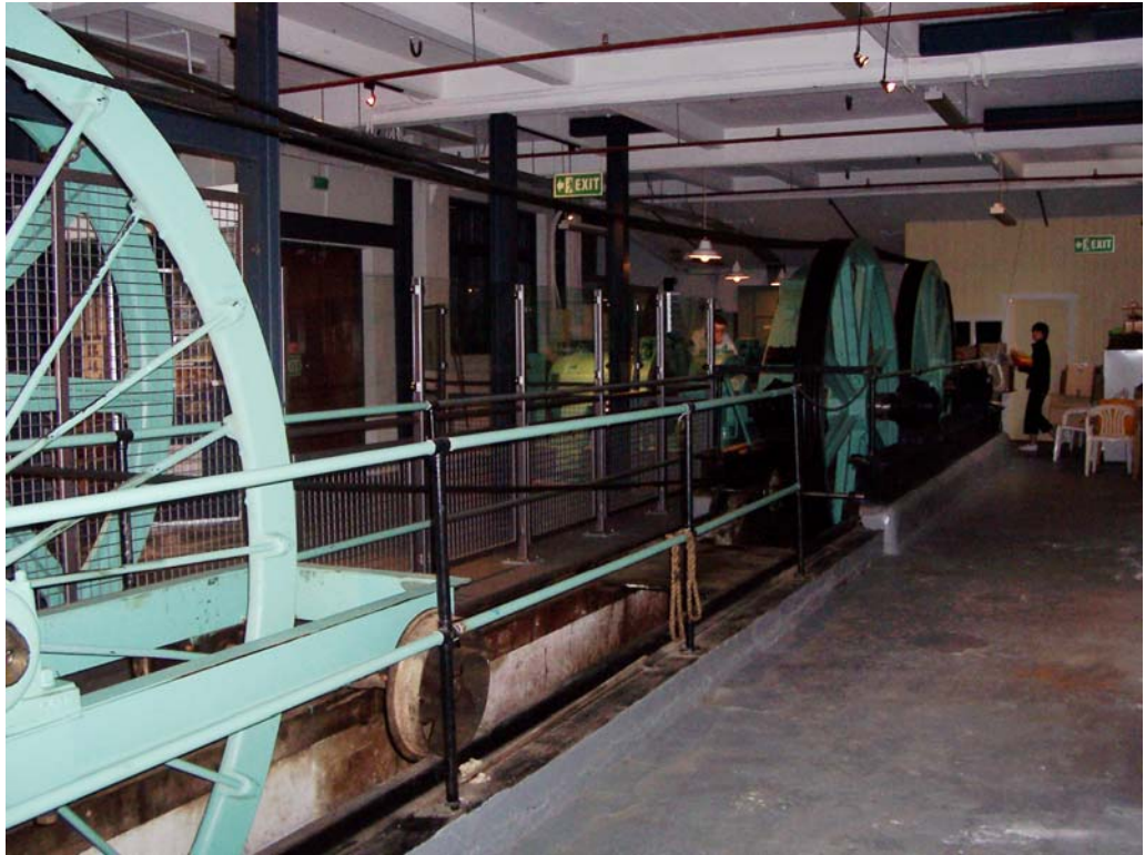
The grip car and trailer behind. Note the sloping seats. The drivers position is behind These seats. Below is the winding gear. In the foreground is the tension wheel and at the far end the idler wheel and the traction wheel.
