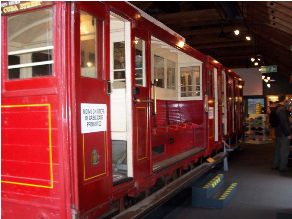
The grip car and trailer behind. Note the sloping seats. The drivers position is behind These seats. Below is the winding gear. In the foreground is the tension wheel and at the far end the idler wheel and the traction wheel.
