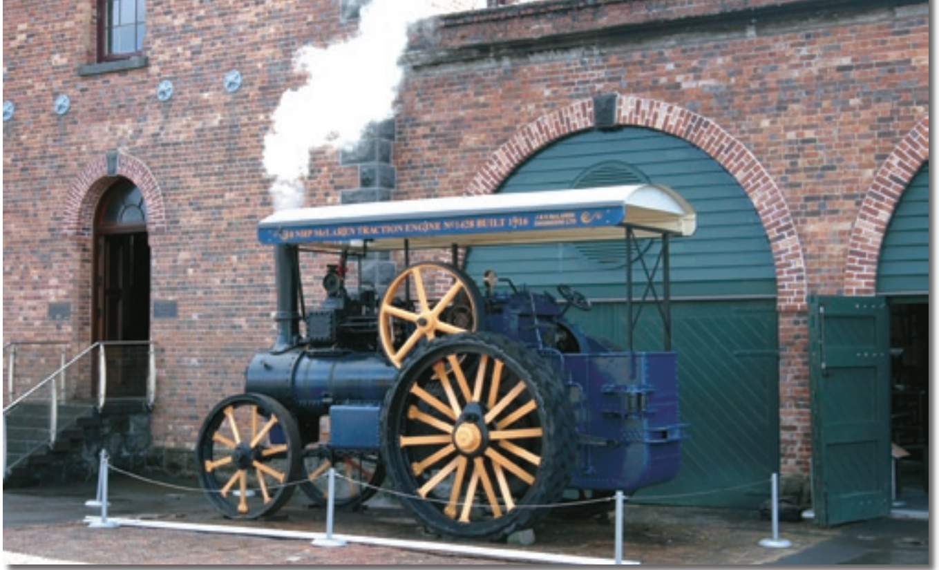
McLaren traction engine under piped steam power.
