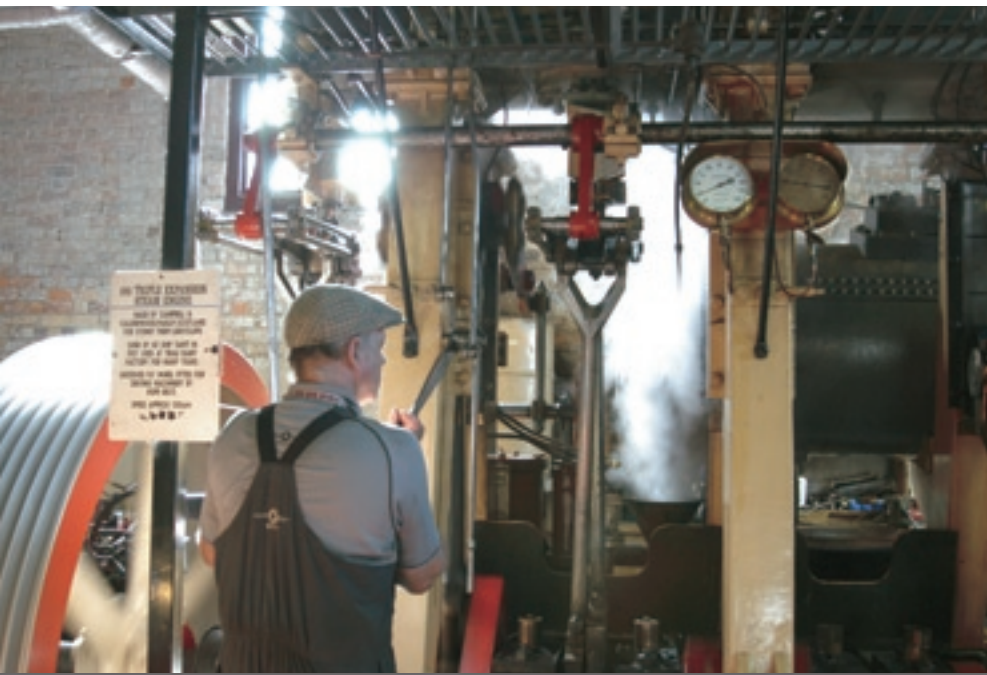
Triple expansion engine from former Sydney ferry. Note grooved flywheel at left.
