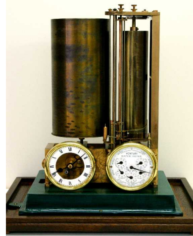
Figure 8 The ex-Waitaki water-flow meter
