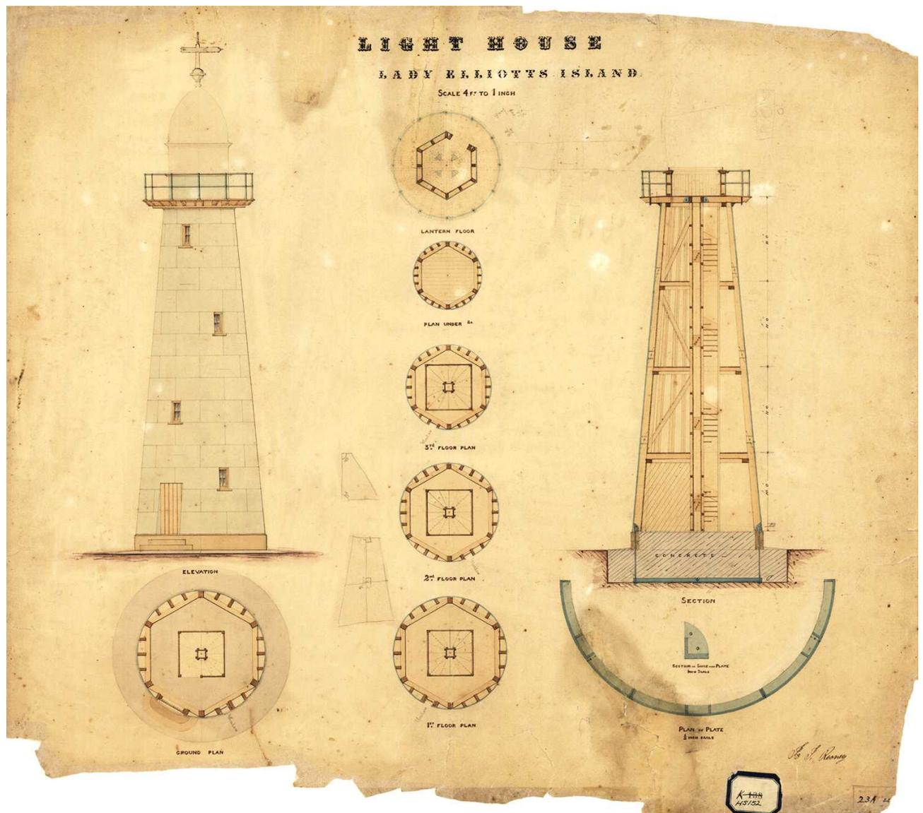
Figure 4. One of the contract drawings for the construction of the Lady Elliot Island lighthouse
