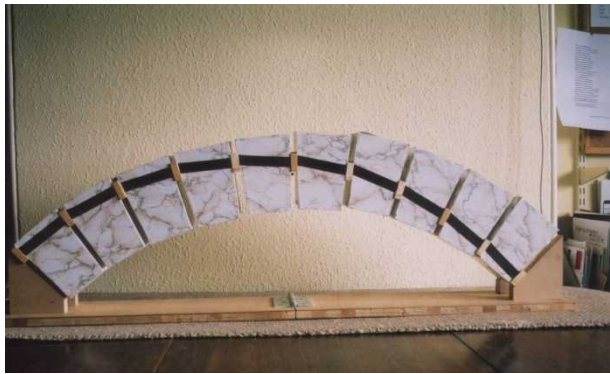
Figure 7 A replica of Barlow's model showing how unpredictable a thrust line is
