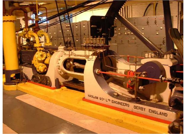
Figure 6: A horizontal open compressor with flywheel.
