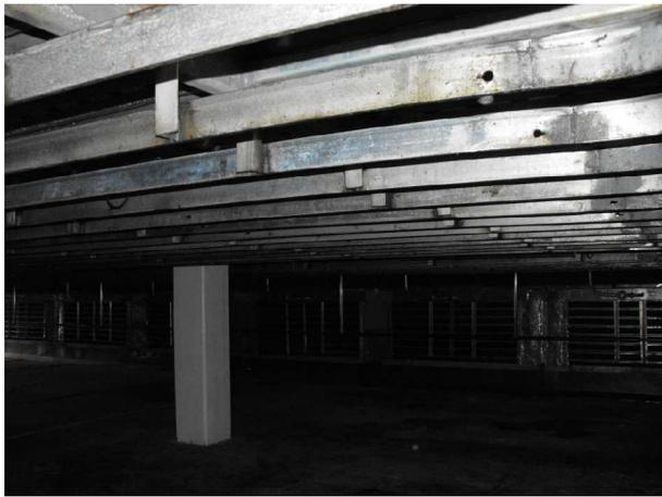
Figure 3: Cross-flow air-blast carcass freezer
